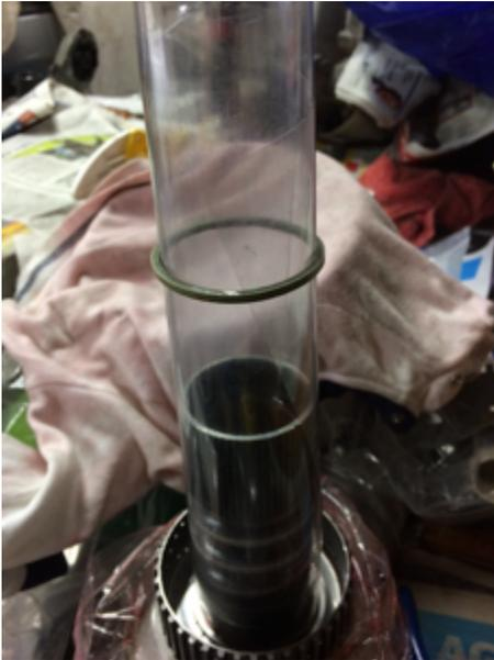
Below shows the extent of the stretch of the seal - I've used the old ones as an example with the correctly sized new ones visible in their grooves.
