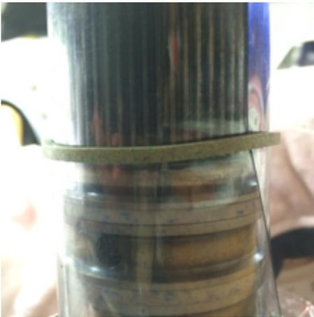
I resized them one at a time starting with fitting the lowest seal first and then fitted the tube over all the seals to compress them. The seals will obviously be loose in the seal groove.
