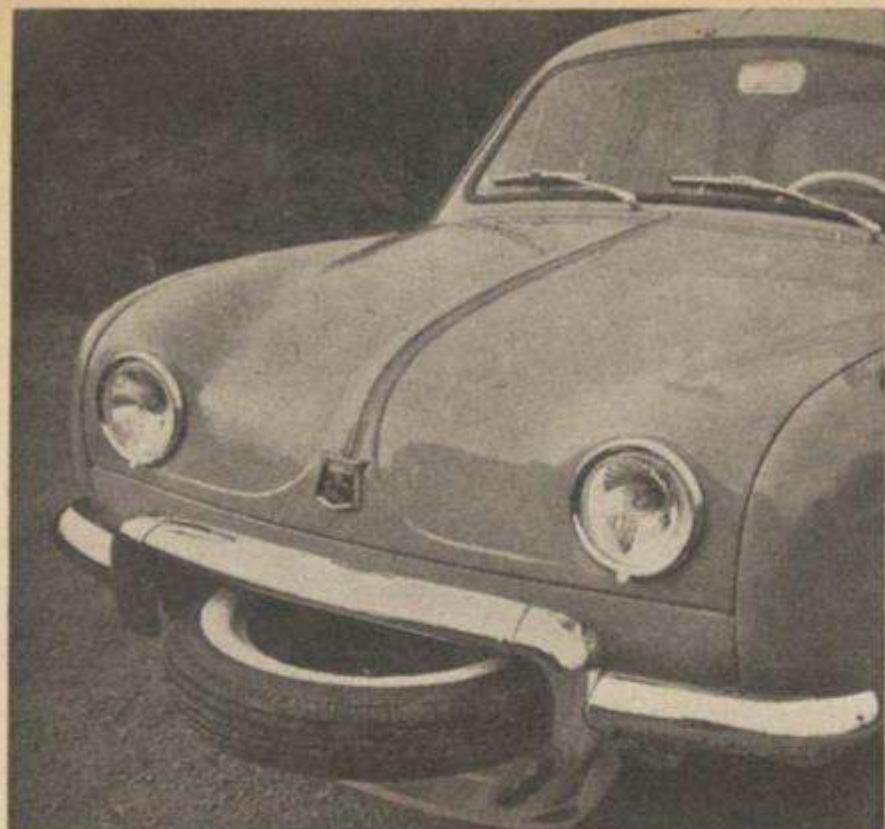
Housing for spare wheel, at front of car, unlocks from inside.
