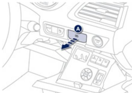
In the event of a failure of the main service brake, a continuous pull on the control lever **A** will stop the vehicle. The dynamic stability control provides stability during emergency braking. If the emergency braking malfunctions, the message "Parking brake control faulty" will be displayed.
