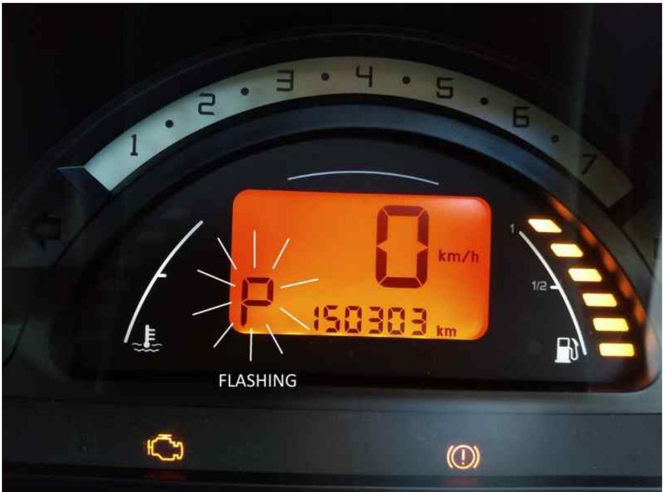
Finally, It's possible that after replacing the ball joint onto the switch arm your gear selector display will flash. If so try re-positioning the switch using the above alignment procedure...again.
