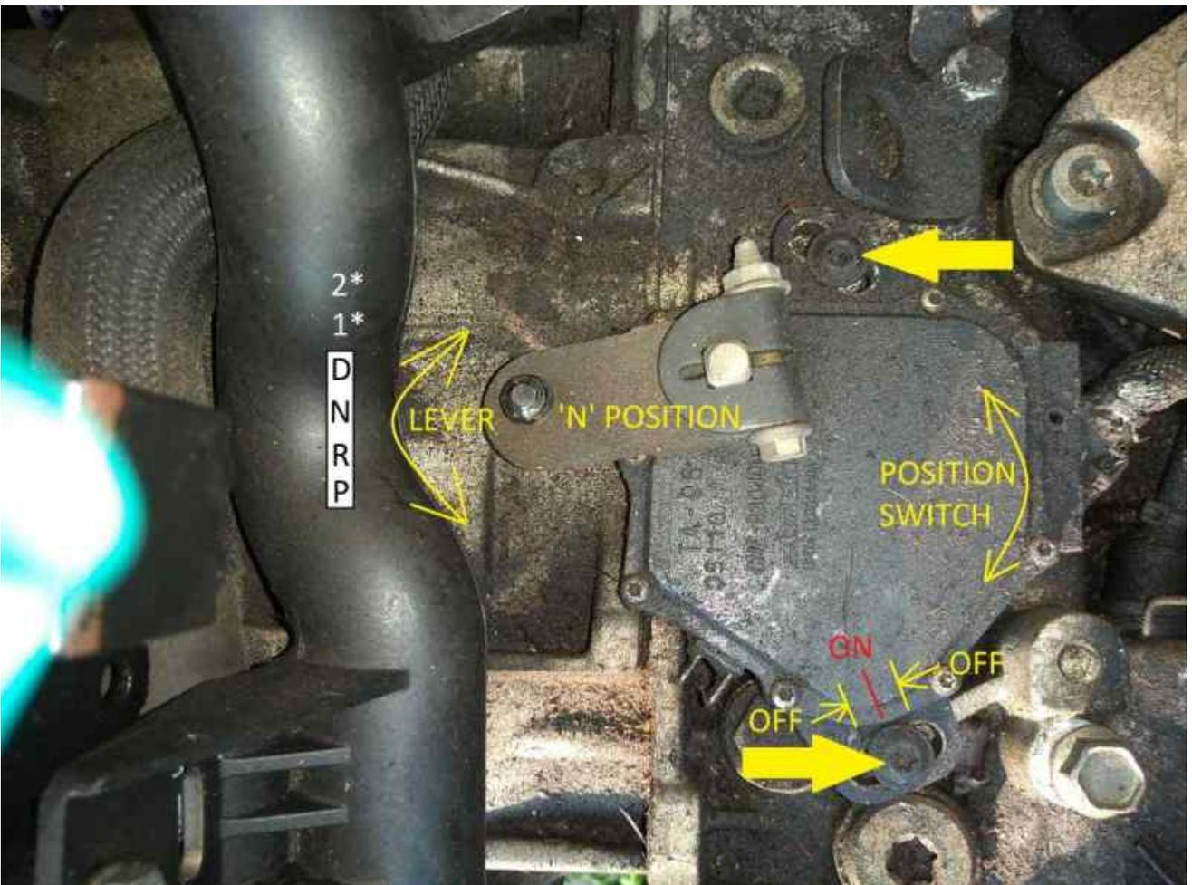
loosen the two retaining screws for the selector switch assembly so it can swivel around the selector arm shaft. Using a mulimeter or some device to check a short circuit, look for continuity across the two exposed contacts on the switch. Move the entire switch backwards and forwards to find the spots where the switch contacts are open circuit (off in the diagram). Find the mid point where there is continuity (on) and lock the two switch retaining screws down.
