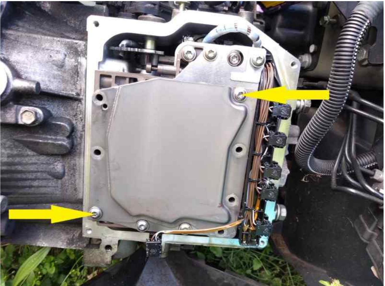
Install the cover and slide 2 of the mounting bolts back into the valve body in positions 4 & 5 .
