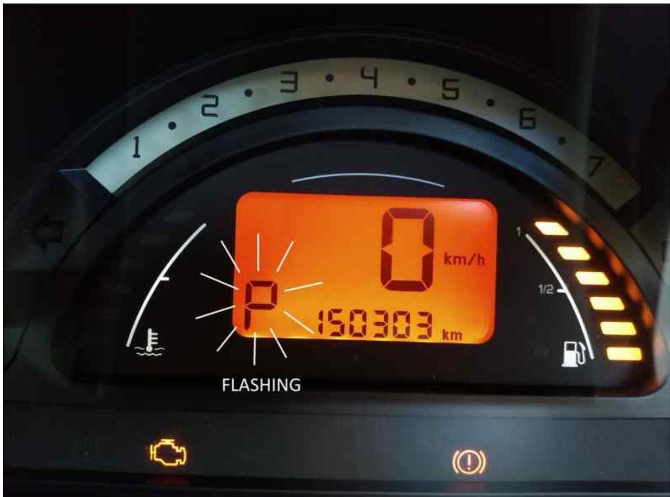
If (later) you put everything back together and the gear selector flashes when some positions are selected, then you will need to continue with the alignment. The quadrant and selector switch are out of alignment.
