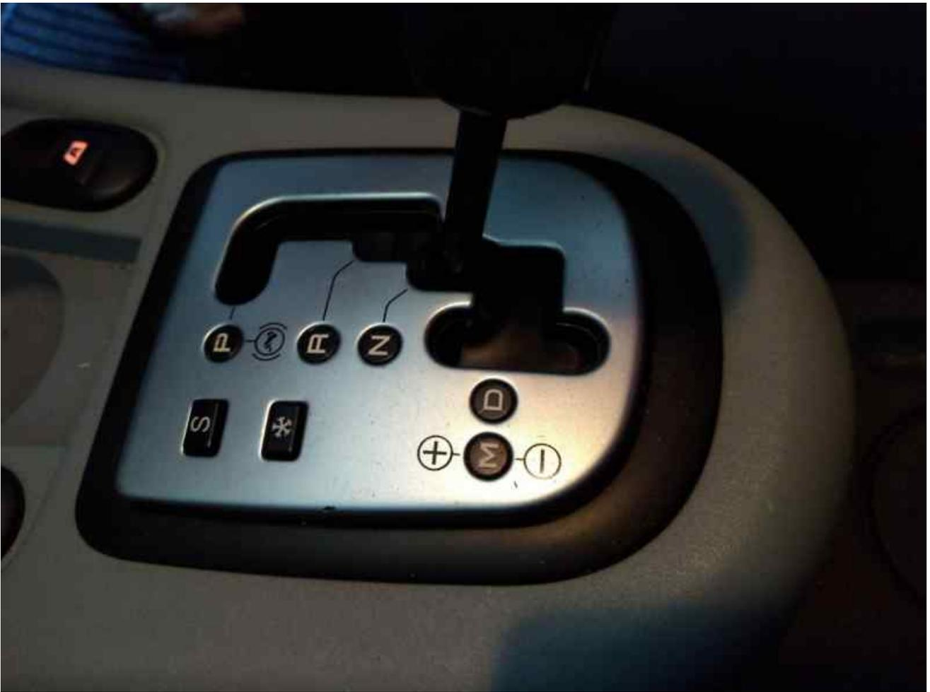
Make sure the gear selector in the cabin is in neutral. If necessary, rotate the selector arm on the transmission to the 'N' position.
