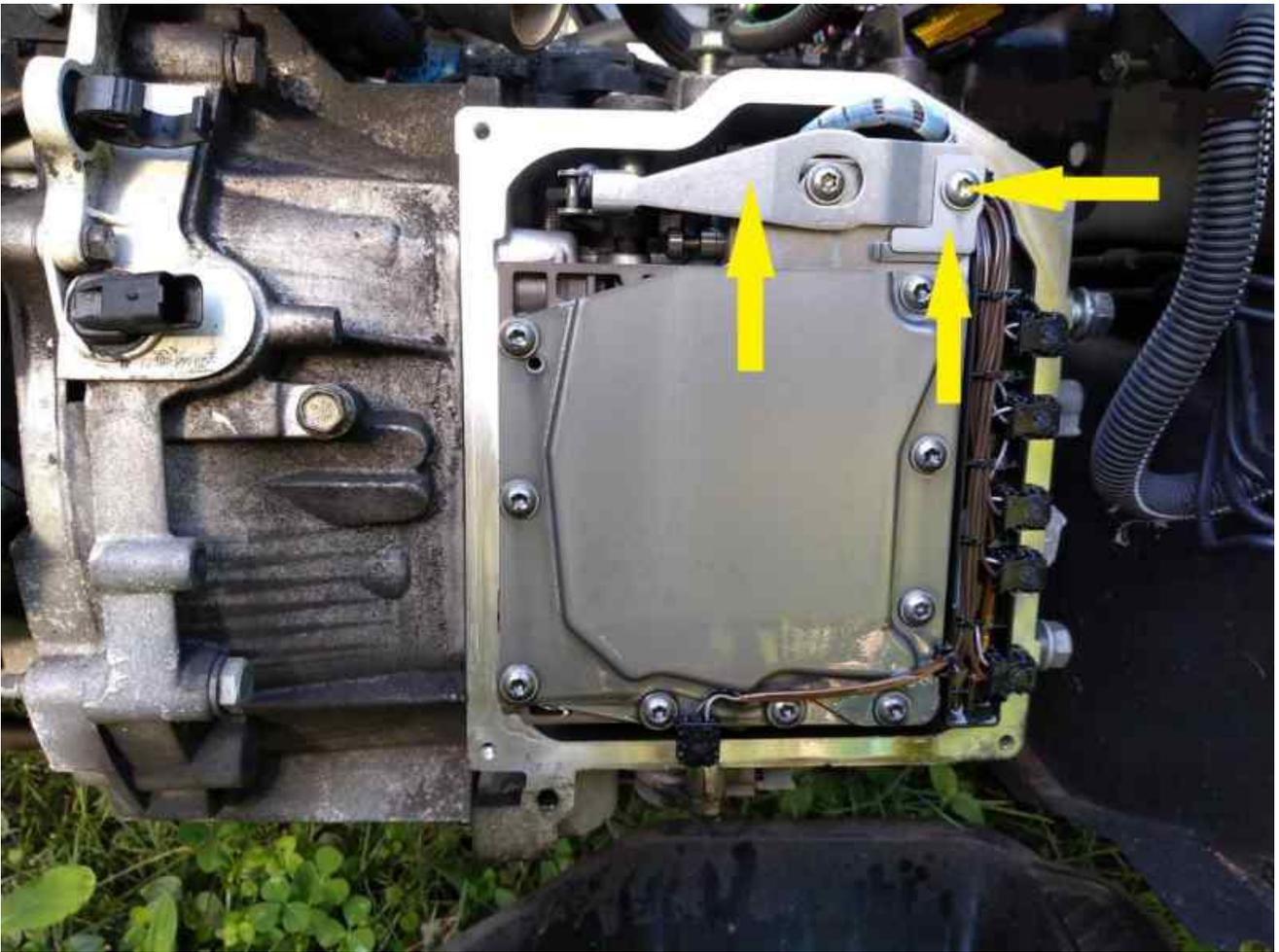
Re-install leaf spring, 'L' shaped washer and retaining bolt. Don't worry where the spring is located at this time and don't fully tighten the retaining bolt.
