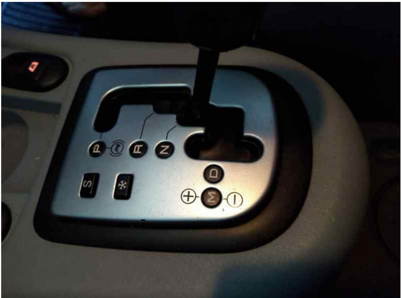
I would recommend disconnecting the battery before proceeding. You will need to perform a BSI reset before and after connecting the battery (search this site). But before doing all that, place the gear selector in the neutral position. Once the battery is removed the selector will be locked if it is left in park. Make sure the hand brake is on and the car can not roll away.
