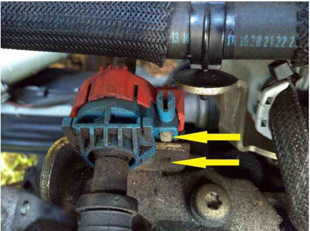
The Bowden cable retainer is held in place by a small clear tab. Pull the pin out while pulling the the retainer upwards off the bracket. The pin is spring loaded. You can now move the entire cable assembly out of your way.
