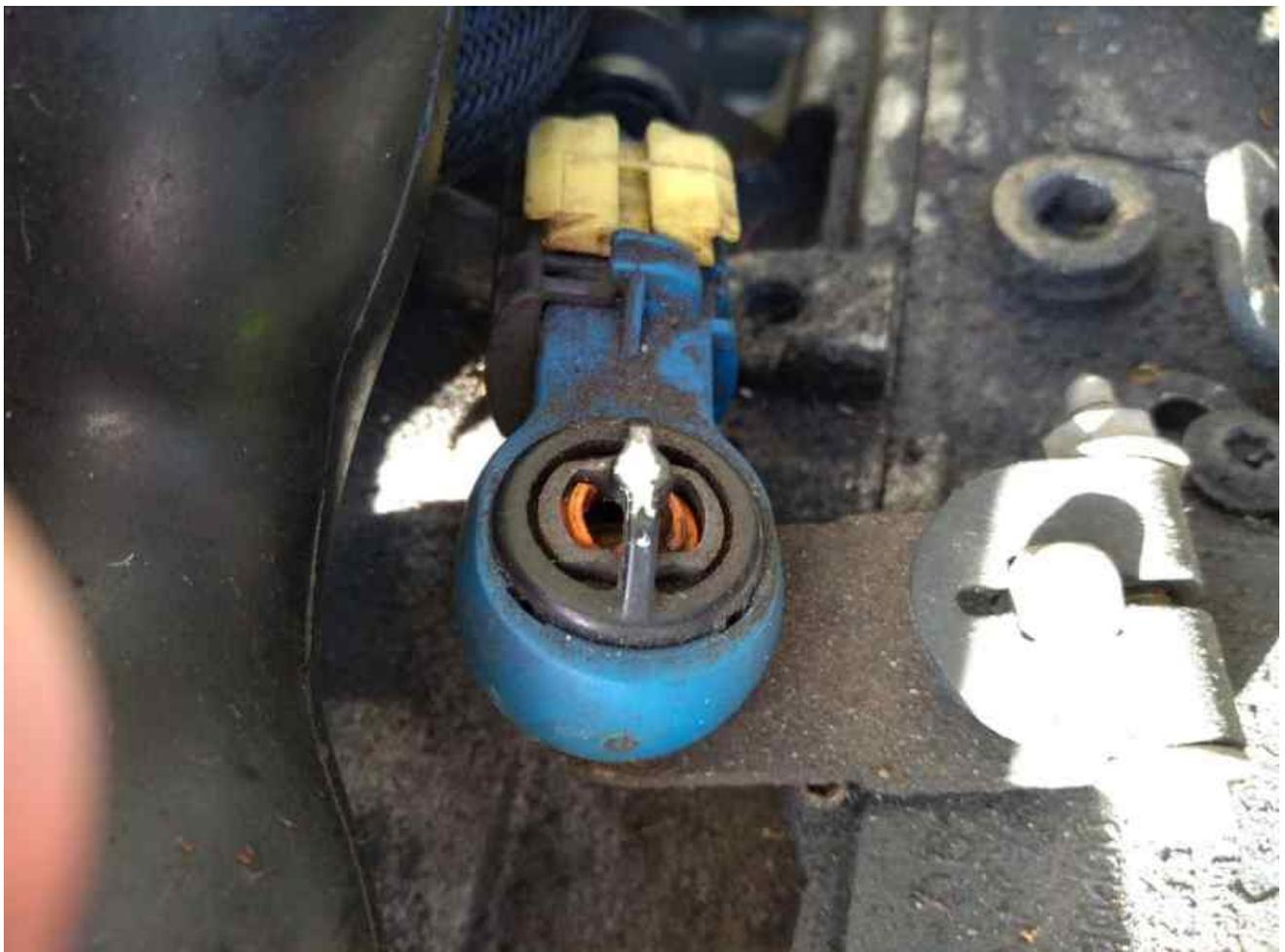
Remove the ball joint connector from the ball joint on the selector switch arm. Press inward on the orange "ears" of the ball joint retainer. Pull upward on the blue rod end while pushing down and inwards on the orange ears.
