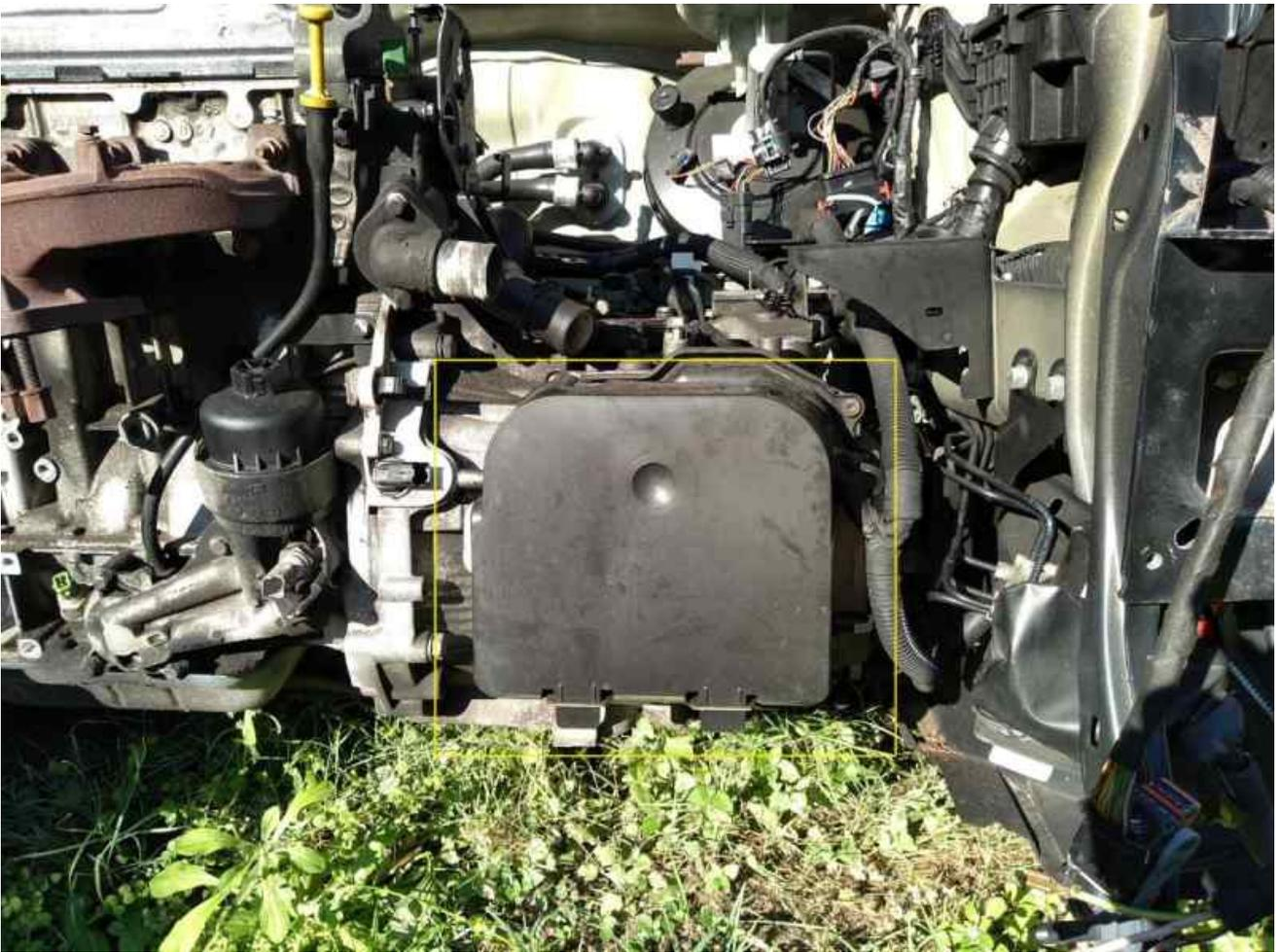
Remove the plastic ECU cover. Then remove the large connector from the top of the ECU. There are 3 cable tie fasteners on the ECU bracket and you need to release the cable from the bracket. I hate these things!! You typically destroy them removing them but the wiring loom needs to be separated from the bracket. You could just let the ECU bracket hang down but it gets in the way.
