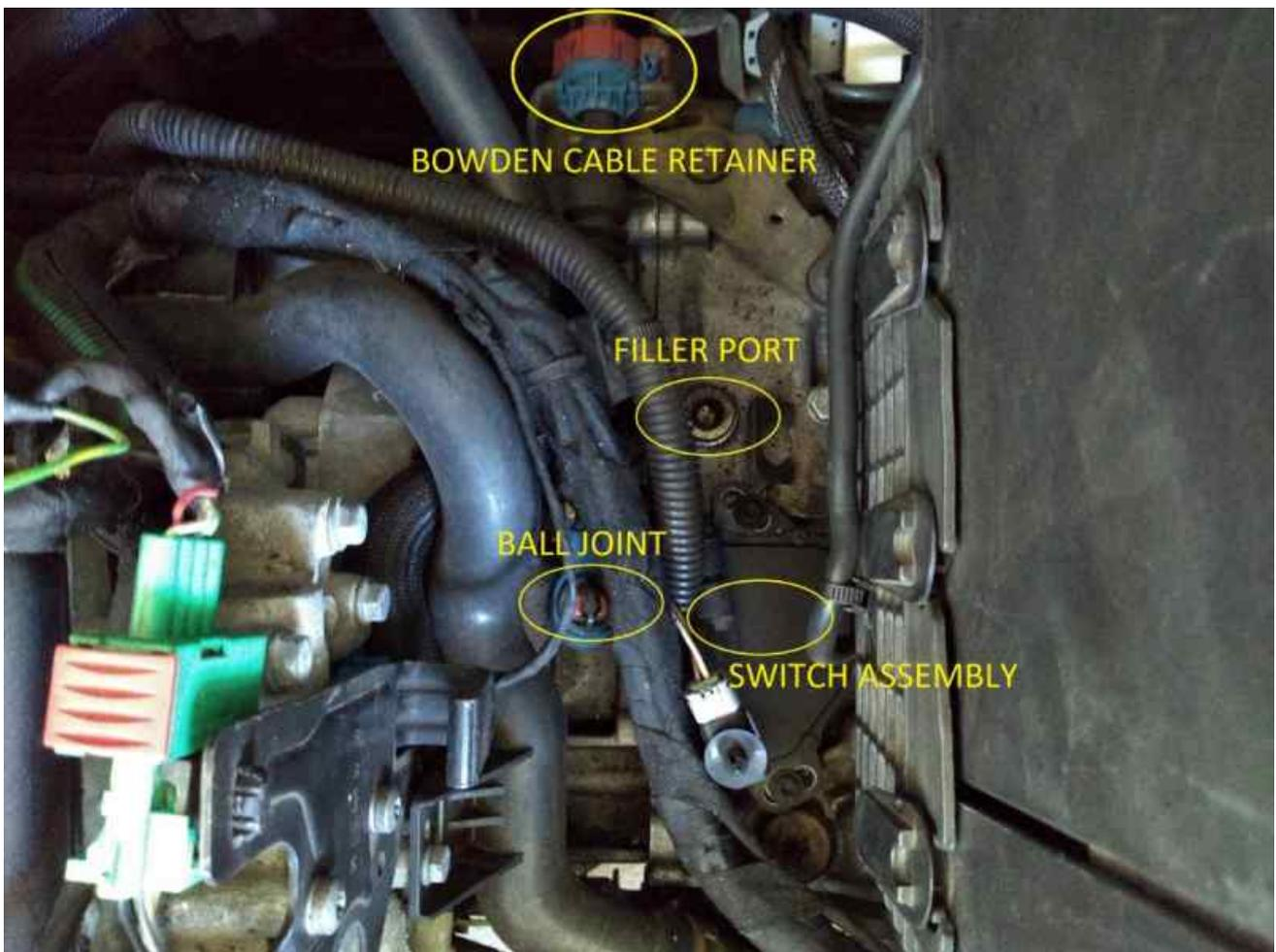
You will (eventually) need to gain access to the oil filler port, the selector cable ball joint, Bowden cable retainer and the selector switch.
