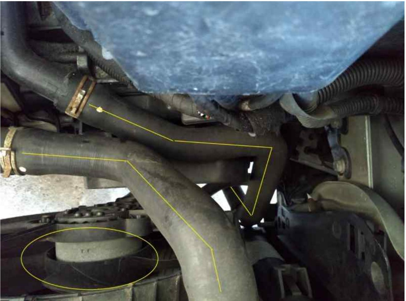
The best way to gain access to the valve body is to remove all the coolant hoses in front of the transmission.
