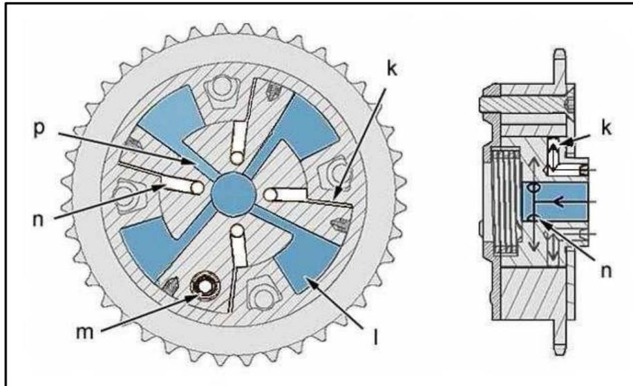
**k:** Camshaft phase shifter chamber.
